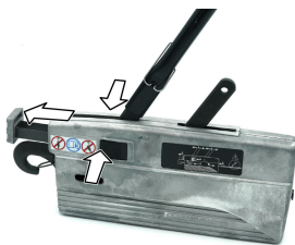
Fig. 3: Release the “Jockey” cable winch
