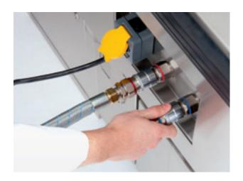
Option: With the Comfort design, the Coolports® can be connected quickly and securely to the conveyor belt's cooling circuit in one hand movement.
