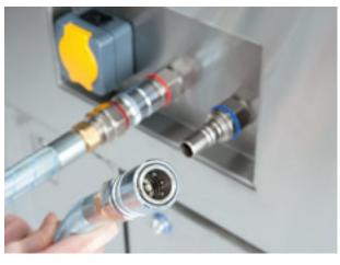
The new quick-release connections make it possible to couple up and uncouple without any tools.
