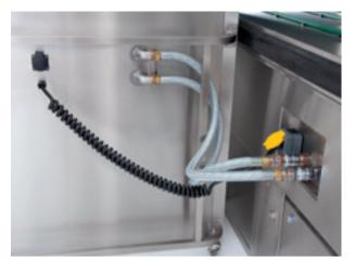
Flexible hose connections enable variable positioning of the Coolports® along the conveyor belt.
