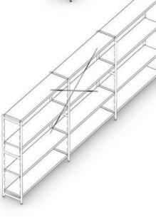
The shelf load is the loading capacity of an individual shelf with a uniformly distributed load.
