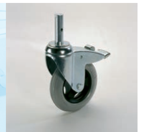
Rust-proof castor with plastic wheel and extremely smooth running surface, ball bearing-mounted in galvanised-chromate housing. This type of castor ensures minimum travel noise and is particularly suitable for running over uneven floors.
