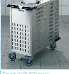
Plate stacker TE-2/VK 19-26 (unheated). Especially suitable for holding portions of cooled food components in Cook & Chill kitchens. The cooling slots ensure rapid exchange of the initially warm stacker atmosphere for the cold air in the cold store and ensure the low temperature is uniformly distributed throughout the crockery. An additional area of use is for the portioning of cold food for distribution in Cook & Serve kitchens.
