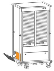
Dust can collect in front of the heat exchanger during operation. Heat exchangers heavily contaminated with dust work inefficiently and consume more energy.
