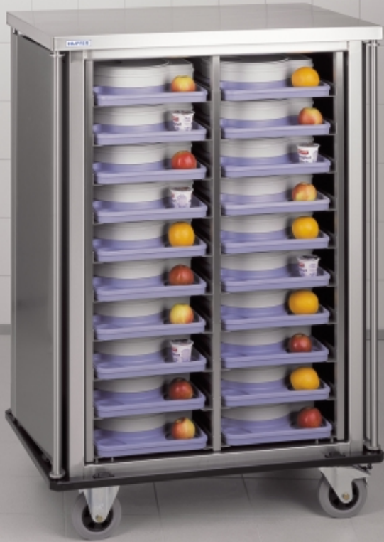
ETTW 2/20 L-EN to hold 530 x 370 mm Euronorm compact trays. The internal space consists of two 10-tray compartments = 20 trays. The trays lie 115 mm apart.
